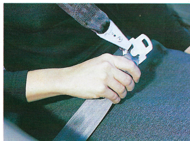
Figure 8 The cloth part of a seat belt does not feel as hot as the metal part.
