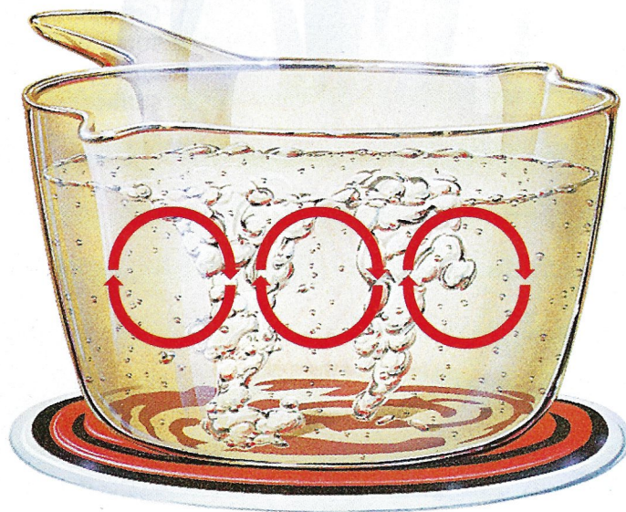
Figure 5 The repeated rising and sinking of water during boiling are due to convection.
